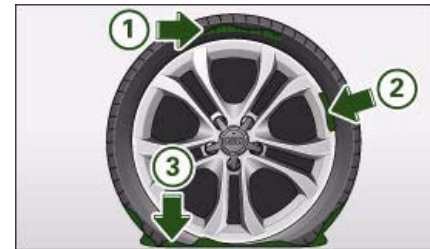
Fig. 227 The Tyre Mobility System is NOT suitable for repairing this type of damage to tyres.
