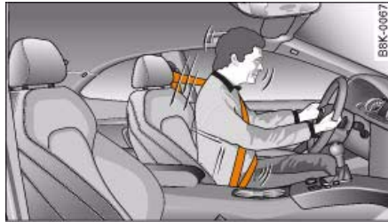
Fig. 166 Driver protected by the properly worn seat belt during a sudden brake manoeuvre
