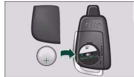
Fig. 128 Remote control: Changing battery
