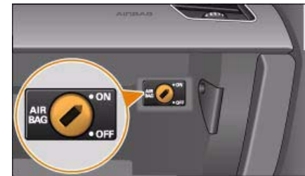
Fig. 184 Key-operated switch in glove box for deactivating front passenger's airbag
