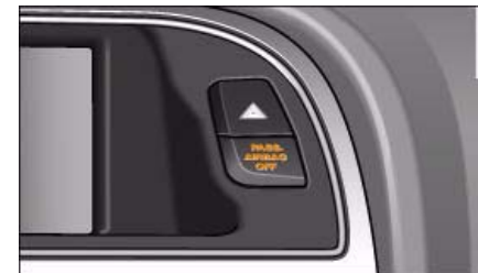
Fig. 185 Lamp indicates that front passenger's airbag has been deactivated via key-operated switch
