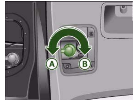
Fig. 245 Diagram: Bulb holder with a bayonet fastener
