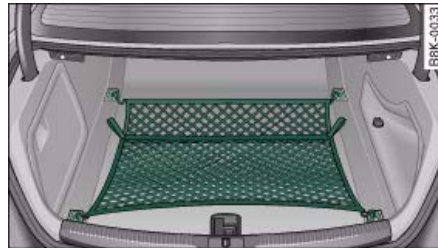
Fig. 81 Stretch net laid out
