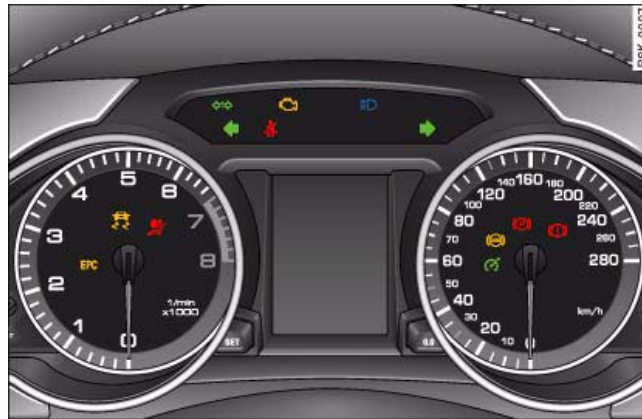
Fig. 7 Instrument cluster with warning and indicator lamps
