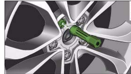
Fig. 233 Changing a wheel: Hexagonal socket in screwdriver handle to turn the wheel bolts after they have been loosened
