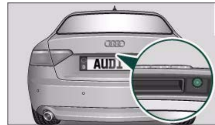
Fig. 143 Boot lid: Location of reversing camera
