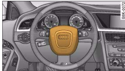
Fig. 176 Driver's airbag in steering wheel
