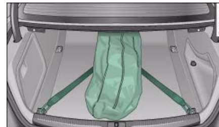
Fig. 90 Luggage compartment: Securing the bag
