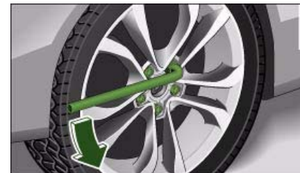
Fig. 230 Changing a wheel: Loosening wheel bolts
