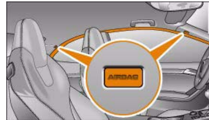
Fig. 182 Location of head-protection airbags above the doors
