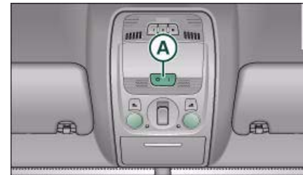
Fig. 57 Headliner: Front interior lights
