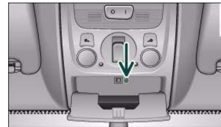
Fig. 48 Detail of headliner: Unscrewing the light housing
