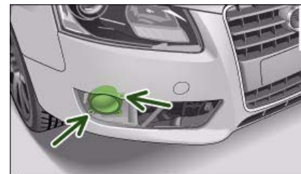
Fig. 249 Screws securing fog light
