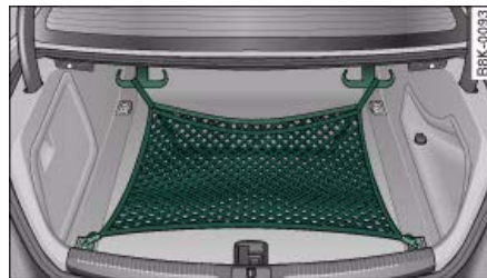
Fig. 82 Stretch net attached in position as retaining net
