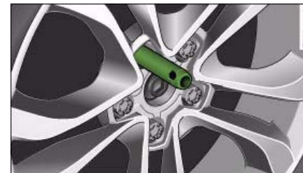
Fig. 234 Changing a wheel: Mounting pin in wheel bolt hole nearest to the top
